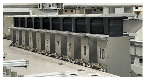
The workpiece clamps are operated as independent interpolation axes. This adopted solution allows further flexibility in the combination of simultaneous work between the different spindles, with the possibility of ensuring a significant increase in production capacity.
